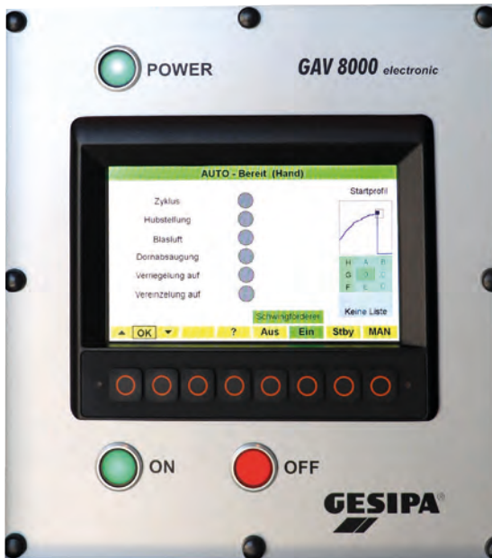
Display of a GAV 8000 electronic indicating the setting curve as part of the setting process monitoring
