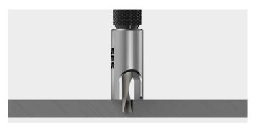
The geometry of the drill hole shall be checked minimum on 1% of all drillings. Nominal measure: Ø 5,9 – 6,0 mm
