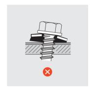
Fastener with sealing washer can only be set correctly by using setting tools equipped with depth locator. Setting with a depth locator results in a uniform setting depth for all fastener.
